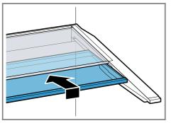
If more space is required, you can fold up the front and rear section of the variable shelf together.
