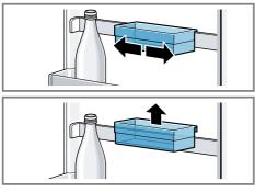
You can remove the door tray rail and re-insert it elsewhere. → "Removing the door tray rail", Page 25
