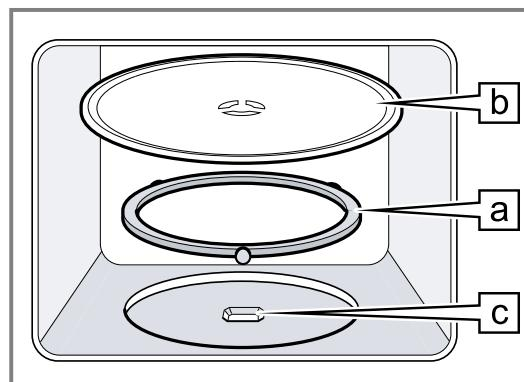
2. Engage the turntable **b** in the drive **c** in the centre of the cooking compartment floor.
