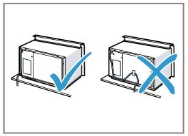
Insert the appliance into the unit and move it to the right.
