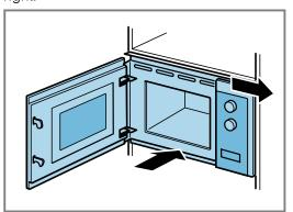
**3.** Screw the appliance in until the appliance is centrally aligned.
