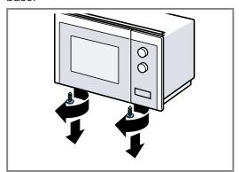
5. Secure the built-in frame on the microwave base with the two outer screws.
