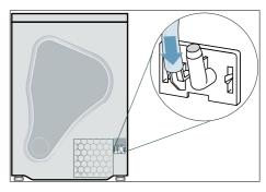
Take the drain hose from the accessories and secure it to the free connecting piece.
