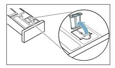
Remove the stopper inserted in the recess on the condensation container.
