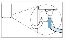
6. Secure the other side of the drain hose using the remaining accessories, depending on the connection situation. Washbasin:
