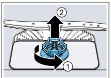
Pull down the micro filter to remove.
