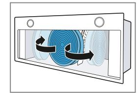
**3.** Carefully slide the odour filter into the holder.
