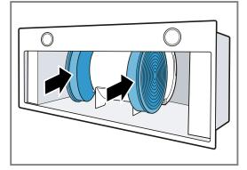
4. Install the grease filters.
