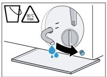
8. Firmly press on the sealing cap.
