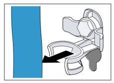
2. Unscrew ① and remove ② all 4 screws for the transit bolts with a WAF 13 wrench.
