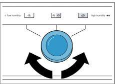
The air humidity in the fruit and vegetable container can be set according to the type and amount of food to be stored by turning the humidity control:
