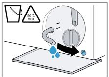
8. Firmly press on the sealing cap.
