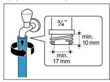
**3.** When connecting to a 21 mm =  $\frac{1}{2}$ " tap, first fit the adapter with a sealing washer.
