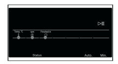
Note: The buttons are sensitive, they only need to be touched gently. If the button Temp. °C \( \begin{align\*} \), rpm \( \end{align\*}, \) Finished in \( \end{align\*} \) is held down, the setting options are automatically scrolled through.
