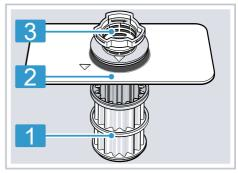
1 Micro filter2 Fine filter3 Coarse filter
