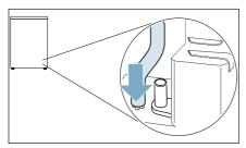
Take the drain hose from the accessories and push it fully onto the free connector.
