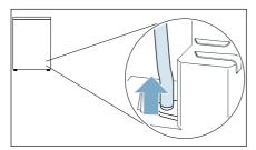
**Note:** The appliance comes delivered with the condensation hose already fitted to the connector.
