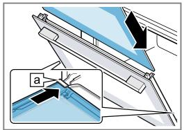
6. Push the inner pane upwards until it is in the leftand right-hand retainers a.
