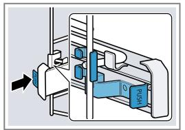
2. Keep the PUSH tab pushed back 1 and swing the rail outwards 2.
