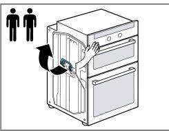
**3.** Place the appliance in the unit and fold the carry handles down.
