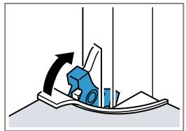
The locking levers are closed. The appliance door is secured and cannot be detached. 4. Close the appliance door.
