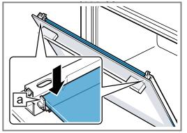
5. Slide the inner pane into the left- and right-hand retainers a.
