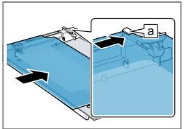
**2.** Push the inner pane upwards until it is in the leftand right-hand retainers a.
