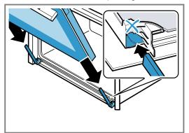
5. Close the locking levers on the left- and right-hand hinges.
