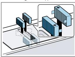
6. Insert the grease filter.
