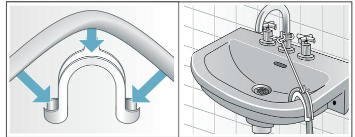
Attach the drain hose securely to the wash basin.
