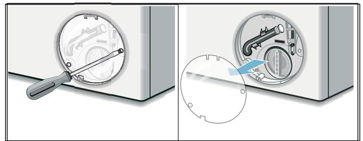
4. Loosen the screws and remove the protective film.
