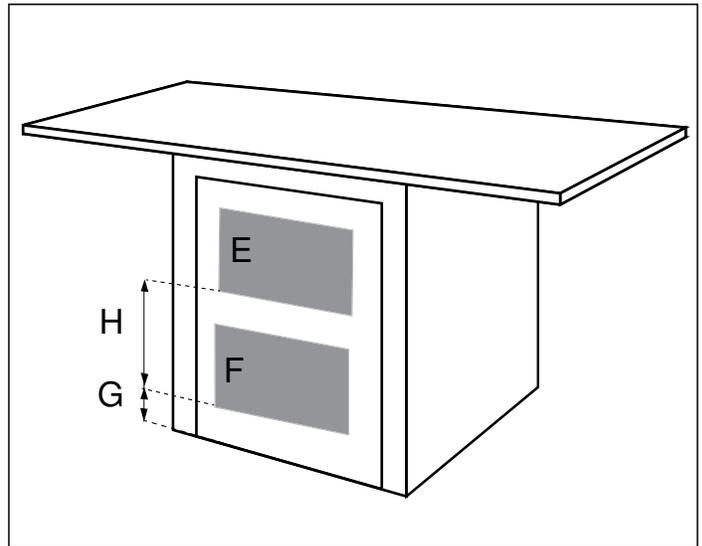
If front of the appliance is covered ventilation openings must be installed.
