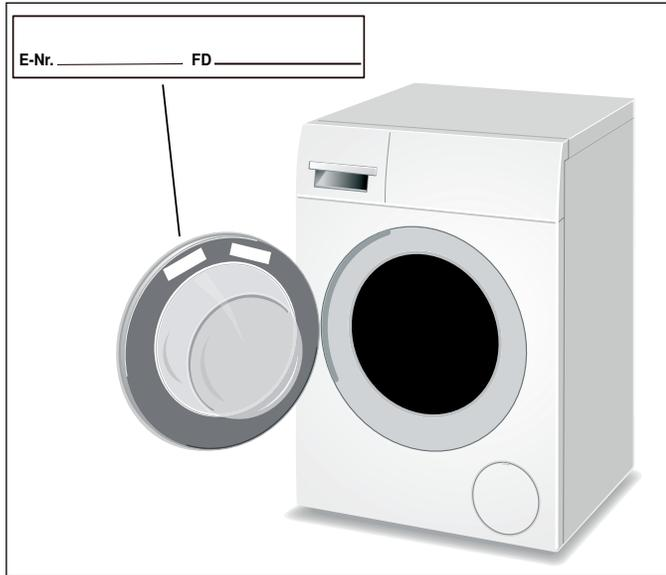
The **E-Nr.** (model number) and the **FD** (serial) number can be found on the rating plate label or in the Home Connect application under Appliance Information.
