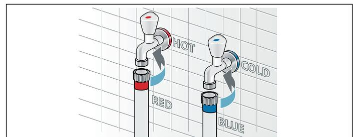
**Attach this end to water tap.** Hand tighten only.
