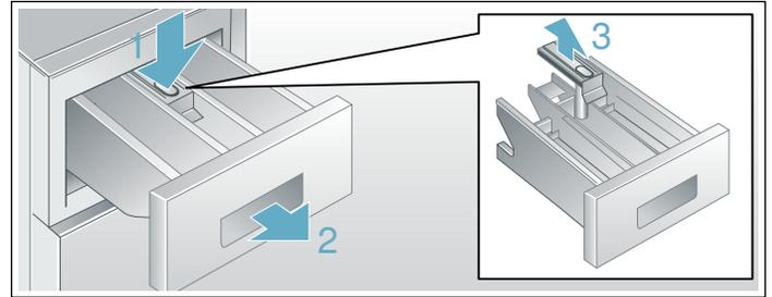
1. Open the detergent dispenser tray fully. Press down on the drawer catch (1) and pull the tray (2) from the washer.
