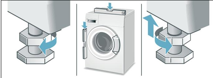
1. After determining which washer feet need to be extended, have someone lift up on the washer slightly to take pressure off the foot to be adjusted.
