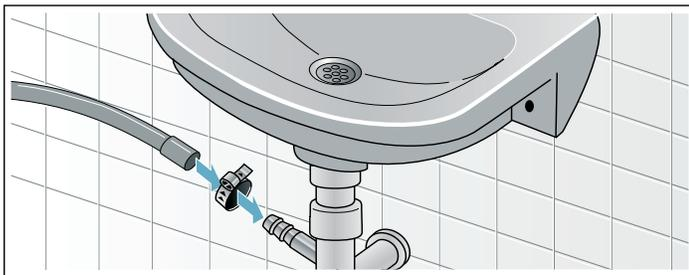
Secure the drain hose to the sink siphon using a  $\varnothing$  0.9 - 1.6 in. (20-44 mm) hose clip (available from a hardware store).
