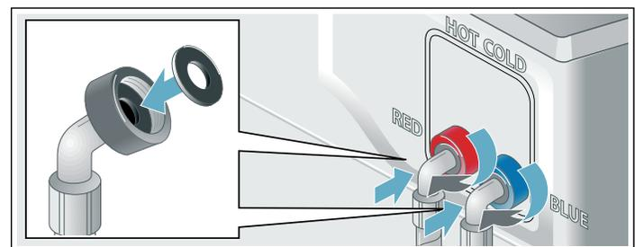
**Attach this end of the hose to the back of the washing machine.** Hand tighten only.
