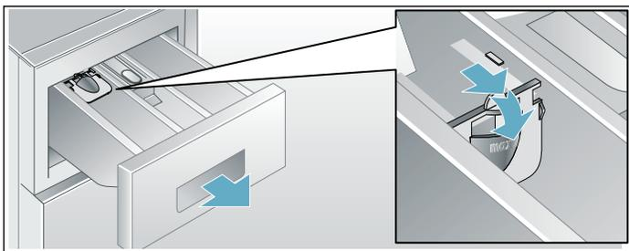
**NOTICE:** Do not use the liquid detergent insert with gel-type detergents and powdered detergents or for cycles with pre-wash or selected "Finish in" time.
