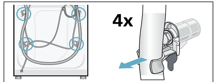
2. Loosen and remove all 4 transport bolts.
