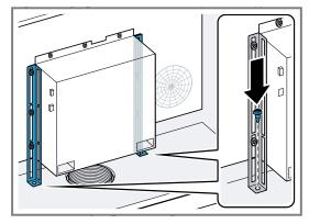
12.Note: If an appliance measuring 90 cm is installed in a unit with a width of 90 cm, skip the next two installation steps and follow the instructions in the additional accessory pack.
