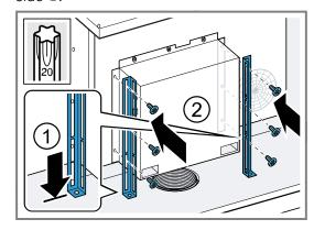
11. Screw the rails onto the bottom of the unit.
