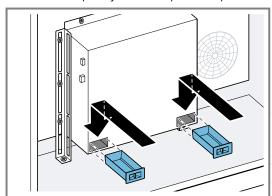
16. Plug the cables into the fan box.
