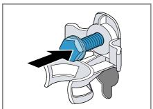
Insert the power cord into the holder ① and tighten all four screws for the transit bolts with a WAF 13 wrench ②.
