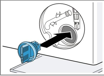
5. Screw on the pump cap.
