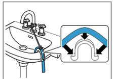
Drainage into a plastic pipe with rubber sleeve or into a gully.
