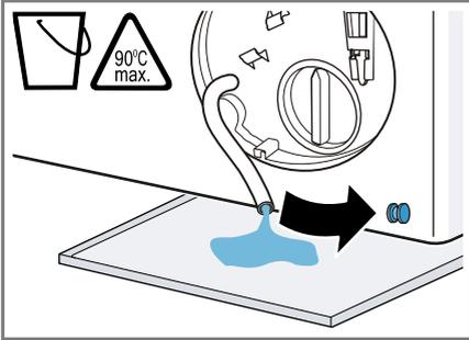
9. Firmly press on the sealing cap.
