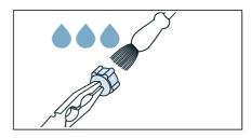
Connect the hose and check for leaks.
