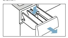
2. To remove the insert: Push the insert upwards from below with your finger.
