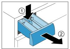
3. Pull out the insert upwards.
