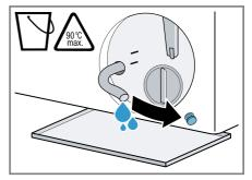
8. Firmly press on the sealing cap.
