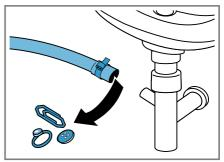
Reattach the water outlet hose and secure the connection point using the hose clamp.
