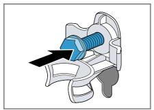
4. Insert the power cord into the holder 1 and tighten all four screws for the transit bolts with a WAF 13 wrench 2.
