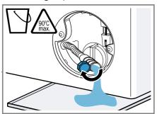
9. Firmly press on the sealing cap.
