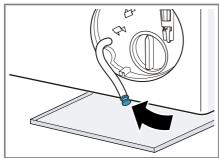
10.Insert the drain hose into the holder.
