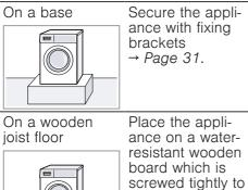
ance on a waterresistant wooden board which is screwed tightly to the floor. The wooden board should be at least 30 mm thick.
