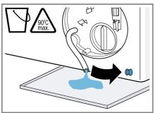
9. Firmly press on the sealing cap.
