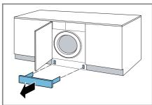
**5.** Slide a sufficiently large receptacle under the opening.
