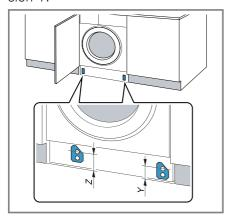
**3.** Screw the spacers in as per the dimensions.
