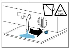
8. Firmly press on the sealing cap.
