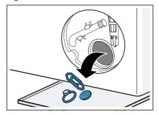
**3.** Make sure that the impeller in the drain pump can be rotated.
