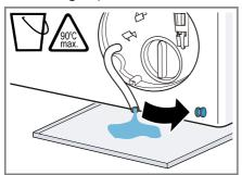
9. Firmly press on the sealing cap.
