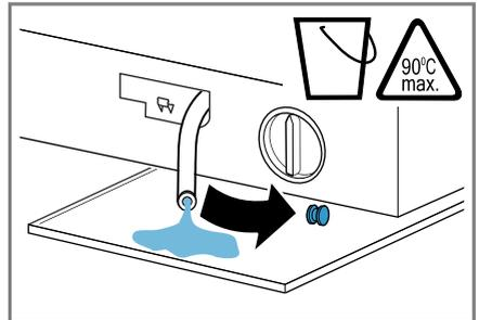
8. Firmly press on the sealing cap.
