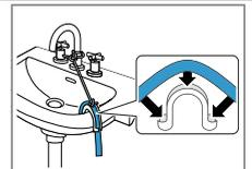
Drainage into a plastic pipe with rubber sleeve or into a gully. Fix and secure the water outlet hose with an elbow.
