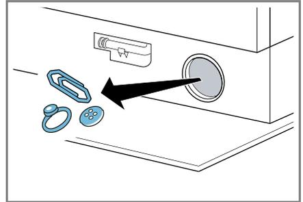
3. Make sure that the impeller in the drain pump can be rotated.
