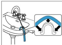
Drainage into a plastic pipe with rubber sleeve.
