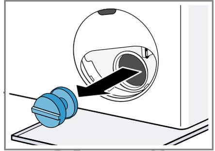
2. Clean the inside and the thread on the pump cap and pump housing.
