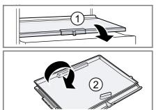
**3.** Press the fastenings for the lower glass plate outwards.
