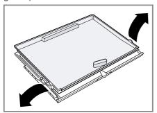
**4.** Lift the glass plate at the front ① and pull it out at the rear ②.
