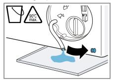
9. Firmly press on the sealing cap.
