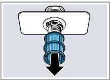
Press the locking catches ① together and lift the coarse filter out ②.
