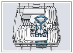
Cutlery basket  $\blacksquare^1$ Large plates up to a diameter of  $31/34 \text{ cm}^1$  can be arranged as shown.
