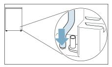
5. Take the drain hose from the accessories and push it fully onto the free connector.
