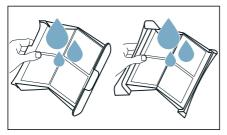
8. Dry the two parts of the fluff filter, snap them shut and reinsert the filter.
