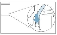
6. Push the drain hose into the appliance's hose guide.
