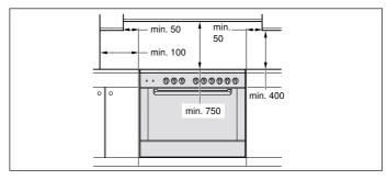
**Note:** Make sure that the distance between the appliance and the back wall is at least 10 mm.
