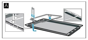
2. Slide the handle onto the rotary spit and screw it on.
