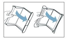
**6.** Remove all fluff from both parts of the filter.
