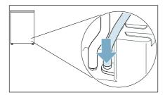
**6.** Push the drain hose into the appliance's hose guide.
