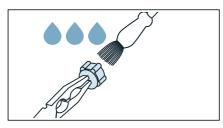
Connect the hose and check for leaks.
