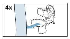
2. Unscrew and remove all four transport brace screws.
