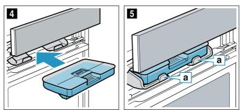
Slowly slide the control panel downwards and then push it towards the rear until it is closed completely. The water tank has been filled. You can start using operating modes with steam.
