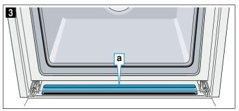
**Note:** If the seal has become detached, fit the seal back onto the drip trough.  $\rightarrow$  "Appliance door" on page 32
