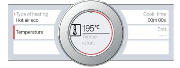
Press the ▷ Start/Stop button to start. The time on the display shows how long the operation has already been running.
