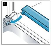
Slide the intermediate glass panel back in and make sure that it is sitting correctly at the bottom in the retainer (fig. 2).
