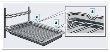
Small steam containers may only be placed in the cooking compartment with the wire rack.
