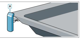
The pull-out rails lock in place when they are fully pulled out. This makes it easy to place the accessories in position.To unlock, push the pull-out rails back into the cooking compartment with a certain amount of force.
