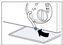
**10.** Insert the drain hose into the holder.
