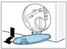
6. Slide a sufficiently large receptacle under the opening.
