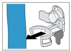
2. Unscrew 1 and remove 2 all four screws for the transit bolts with a WAF 13 wrench.
