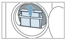
**3.** Remove the fluff from the fluff filter recess. Ensure that no fluff falls into the open shaft.
