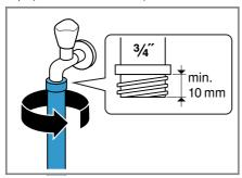
Open the water tap carefully and check that the connection points are tight.
