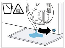
9. Firmly press on the sealing cap.
