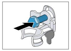
4. Insert the power cord into the holder ① and tighten all four screws for the transit bolts with a WAF 13 wrench 2.
