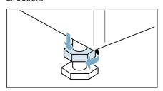
Check the alignment of the appliance with a spirit level, and adjust it if necessary. Change the height by turning the appliance feet. All four appliance feet must stand firmly on the ground.
