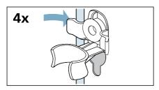
b) Insert and tighten the screws.
