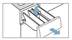
To remove the insert: Push the insert upwards from below with your finger.
