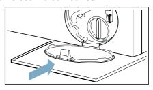
**Note:** To prevent unused detergent from flowing straight into the drain during the next wash: Pour 1 litre of water into manual dosing compartment and start the **Prain** programme.
