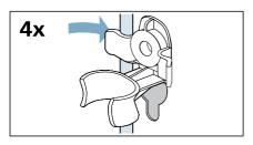
b) Insert and tighten the screws.
