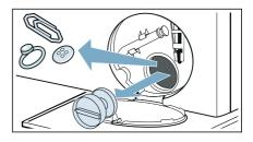
Refit and screw on the pump cover. The handle must be in a vertical position.
