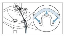
Drainage into a plastic pipe with rubber bushing or into a drainage pit
