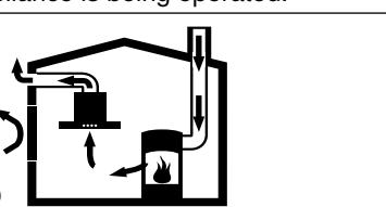
Room air-dependent heat-producing appliances (e.g. gas, oil, wood or coal-operated heaters, continuous flow heaters or water heaters) obtain combustion air from the room in which they are installed and discharge the exhaust gases into the open air through an exhaust gas system (e.g. a chimney).
