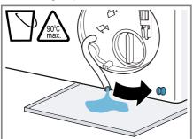
9. Firmly press on the sealing cap.
