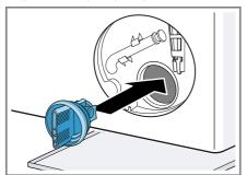
Make sure that the components of the pump cap are securely seated.
