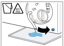
9. Firmly press on the sealing cap.
