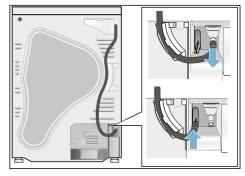
Take the drain hose from the accessories and secure it to the free connecting piece.
