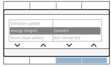
Your appliance now attempts to connect to the smart energy system (energy manager). If the appliance has connected successfully, **Connected**  $\checkmark$  appears in the display.
